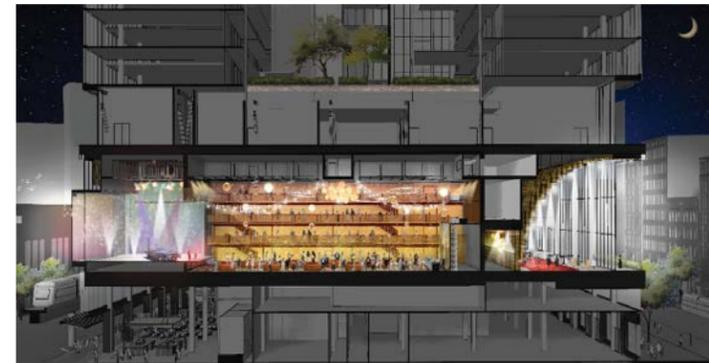
Figure 12. Illustration of Convertible Hall in flat-floor mode
